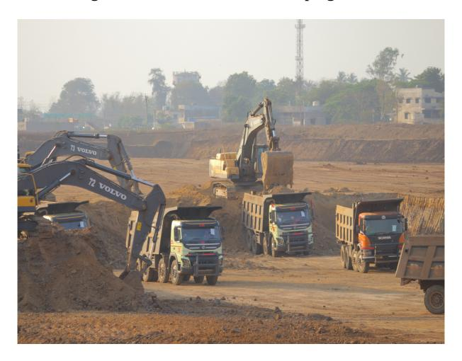
The mine has total 48.92 million tonnes Geological reserves out of which 33.90 million tonnes is can be mine which is excavated through Opencast Mining using Hydraulic excavators and dumper combination along with ancillary equipment such as Dozer, Water Sprinkler, Motor Grader etc.
