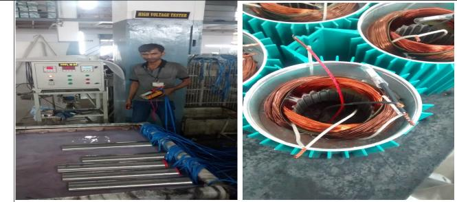
we have seen testing department, their check motor on no load and loading condition. They take reading, how much ampere current drawn by motor, how much LPS water pumping and height of head.
